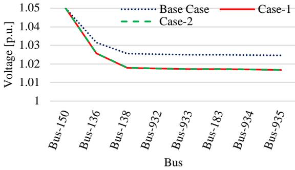
Figure 21. Voltage profile of the line from slack Bus-150 to EV Bus-935
