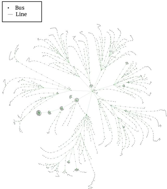
**Figure 4. Network topology of the 1536-Bus real distribution system provided by the distribution system operator in Türkiye for a 2023 case<sup>14</sup>**
