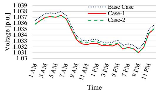
Figure 12. Voltage profiles of the bus connected to the high-level DC charger
