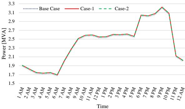
Figure 6. Loading profiles of the line connected to the medium-level AC charger bus
