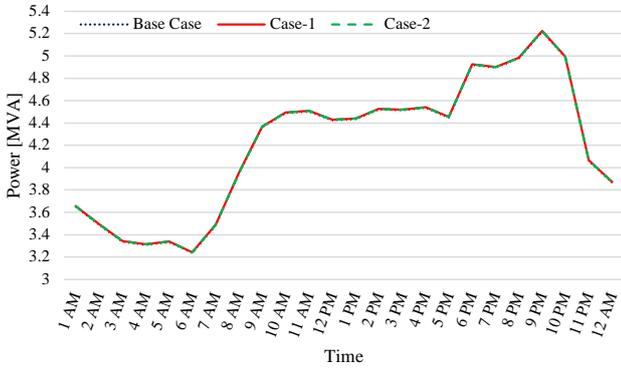
Figure 5. Loading profiles of the line connected to the low-level AC charger bus
