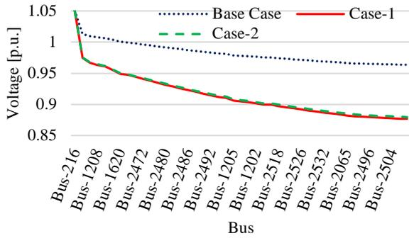
Figure 31. Voltage profile of the line from slack Bus-216 to EV+DG Bus-2508
