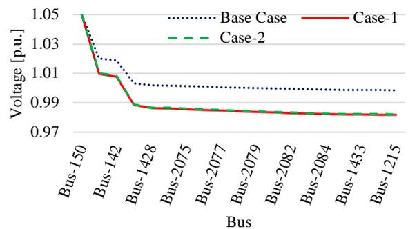
Figure 20. Voltage profile of the line from slack Bus-150 to EV Bus-1215
