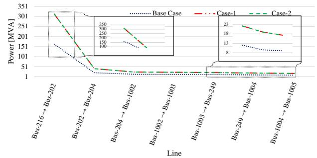
Figure 25. Feeder load flow from the slack Bus-216 to EV Bus-1005
