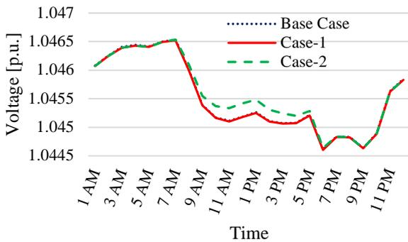
Figure 14. Voltage profiles of the bus connected to the 920-kW DG
