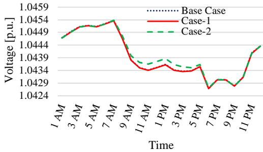
Figure 13. Voltage profiles of the bus connected to the 240-kW DG
