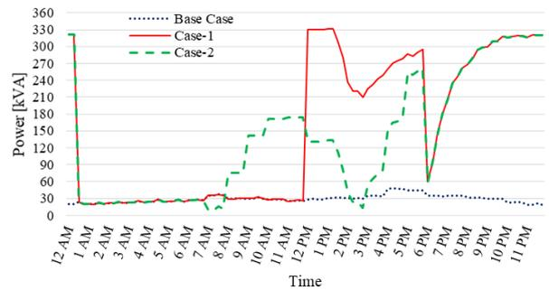
Figure 39. Loading profiles of the line connected to the bus with 100 EVs, HP load, and a 200-kW installed-capacity PVP
