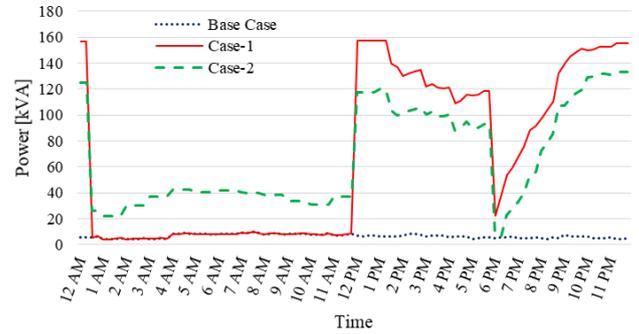
Figure 38. Loading profiles of the line connected to the bus with 50 EVs, a HP load and a 50-kW installed-capacity WPP
