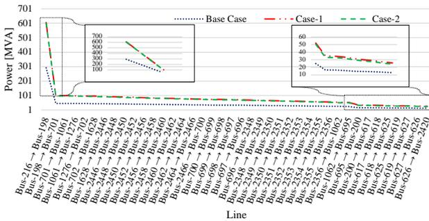
Figure 28. Feeder load flow from slack Bus-216 to EV+DG Bus-2420
