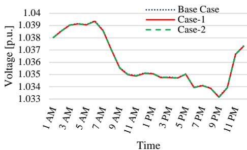
Figure 10. Voltage profiles of the bus connected to the low-level AC charger
