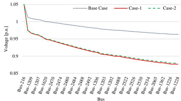
Figure 30. Voltage profile of the line from slack Bus-216 to EV+DG Bus-1228
