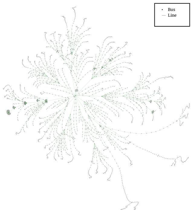
Figure 24. Projected network topology of 2550-Bus distribution system provided by distribution system operator in Türkiye for 2038 case
