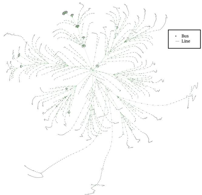
Figure 15. Projected network topology of the 2152-Bus distribution system provided by the distribution system operator in Türkiye for the 2030 case<sup>16</sup>
