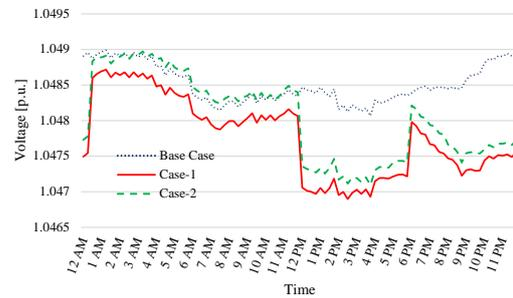
Figure 40. Voltage profiles of the buses with 50 EVs, a HP load and a 50-kW installed-capacity WPP
