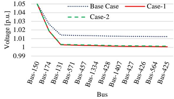
Figure 23. Voltage profile of the line from slack Bus-150 to EV+DG Bus-425
