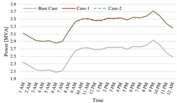
Figure 7. Loading profiles of the line connected to the high-level DC charger bus
