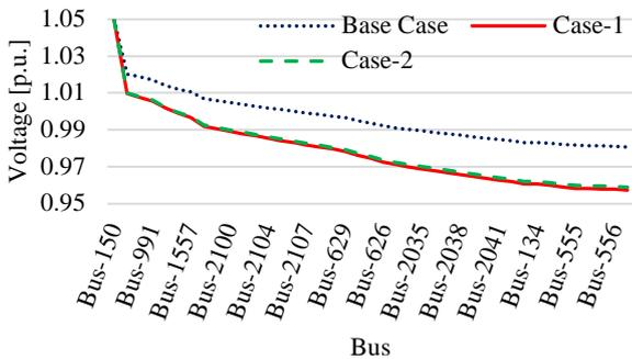
Figure 22. Voltage profile of the line from slack Bus-150 to EV+DG Bus-2085
