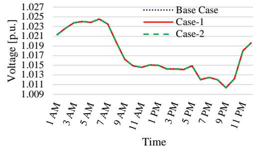
Figure 11. Voltage profiles of the bus connected to the medium-level AC charger
