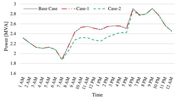
Figure 8. Loading profiles of the line connected to the 240-kW DG bus
