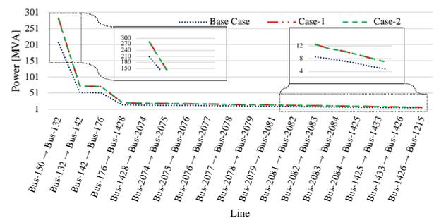
Figure 16. Feeder load flow from slack Bus-150 to EV Bus-1215
