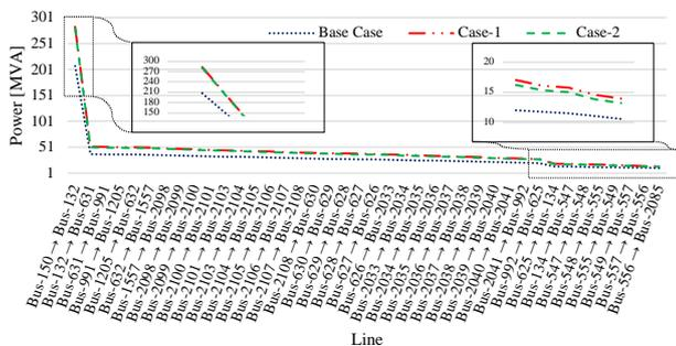
Figure 18. Feeder load flow from slack Bus-150 to EV+DG Bus-2085
