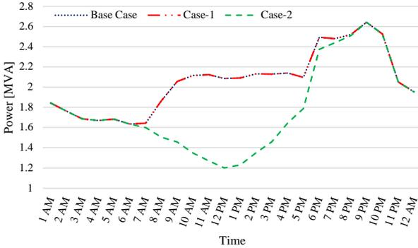
Figure 9. Loading profiles of the line connected to the 920-kW DG bus
