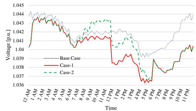
Figure 41. Voltage profiles of the buses with 100 EVs, a HP load and a 200-kW installed-capacity PVP
