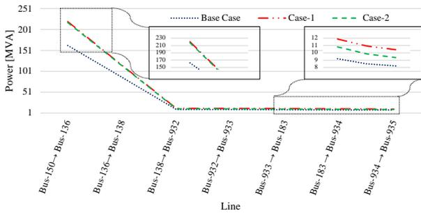
Figure 17. Feeder load flow from the slack Bus-150 to the EV Bus-935
