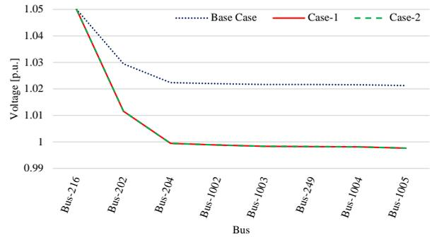
Figure 29. Voltage profile of the line from slack Bus-216 to EV Bus-1005
