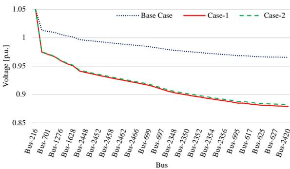
Figure 32. Voltage profile of the line from slack Bus-216 to EV+DG Bus-2420
