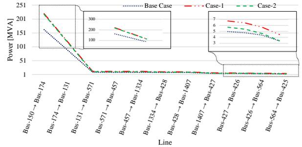
Figure 19. Feeder load flow from slack Bus-150 to EV+DG Bus-425
