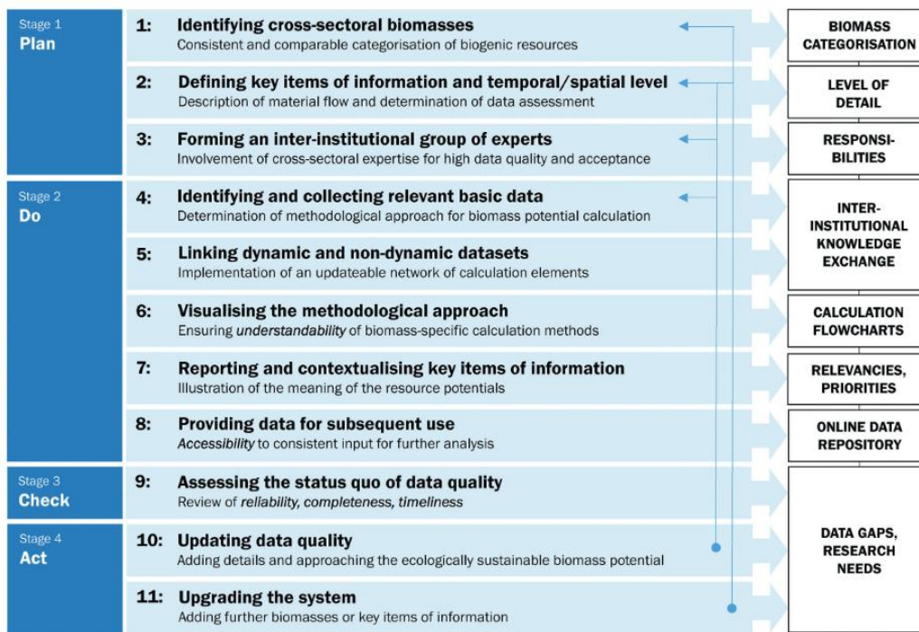
Figure 6: Implementation process for the monitoring system 15
